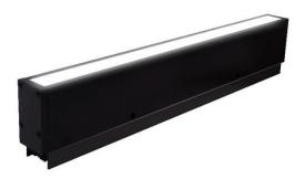
Utilizing a full rod focal lens, the UL-LL provides a tight structured beam of light up to 12 inches (30.48 cm). The optimal working distance is 5 inches (12.7 cm). For working distances beyond 12 inches (30.48 cm), please see our Collimated Line Light offerings. High uniformity (±5%) makes the UL Line Light ideal for front and back lighting line scan applications.
